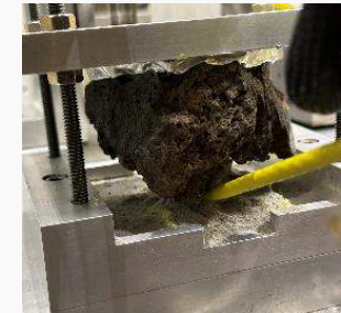
Abrasion testing of tether in Lunar thermal environment
