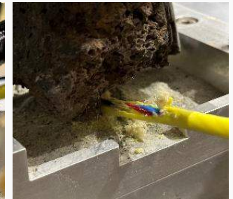
Abrasion testing of tether in Lunar thermal environment
