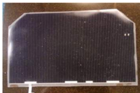
Image of Spectrolab ITJ cell covered with fused silica PMG 1
