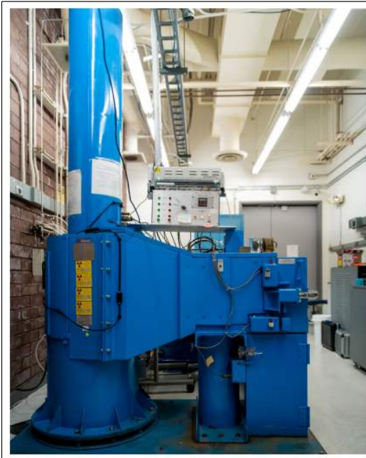
Gamma testing: Co-60 radiator
