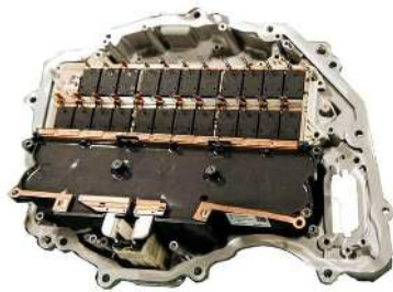
SiC based Dc/Ac traction drive inverter in Tesla Model 3
