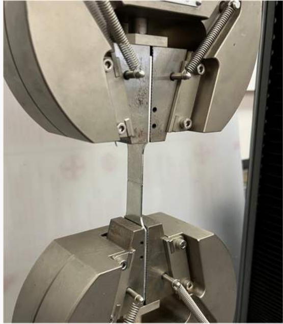
Instron pull testing
