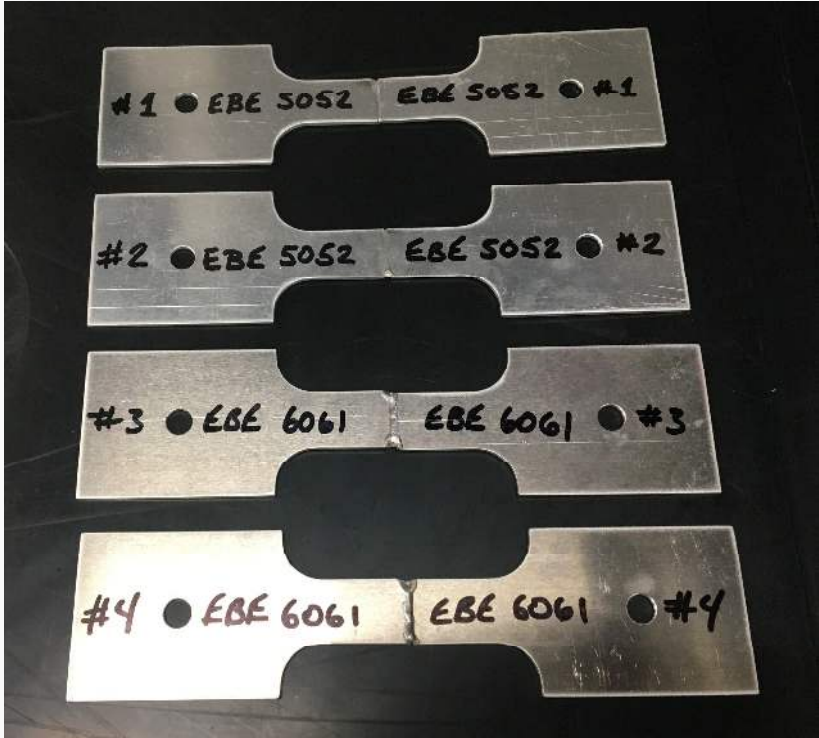
Laser welded test coupons (5052 and 6061 alloys)
