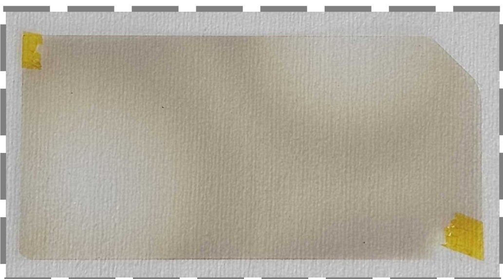
MgF 2 after atomic oxygen exposure
