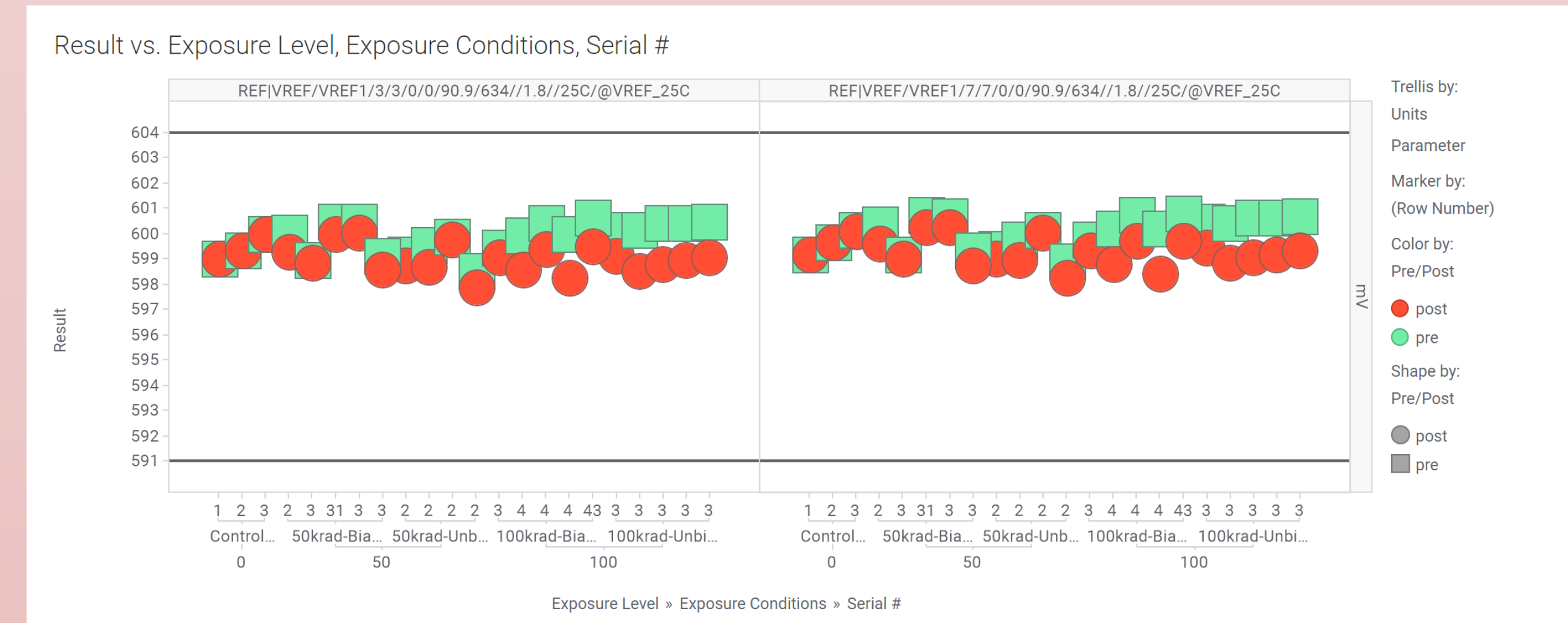
Fig. 4 Internal Voltage Threshold Performance vs HDR levels
