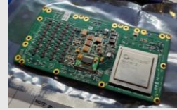
Motor Control Board
