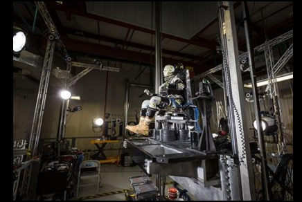
Vertically Accelerated Load Transfer System
