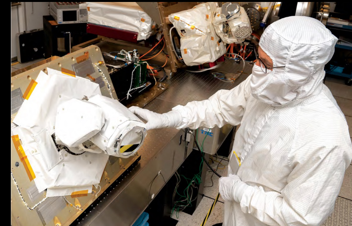
Optical comms terminal Illuma-T built to greatly accelerate data transmission from ISS Credit: MIT Lincoln Laboratory
