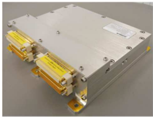
Provide panel to panel fault isolation, power and EMI filtering of SA power
