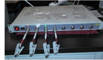
Battery Test Stations
