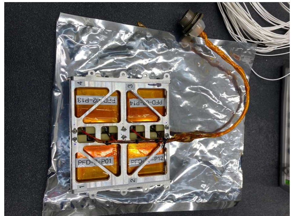
4s1p battery module
