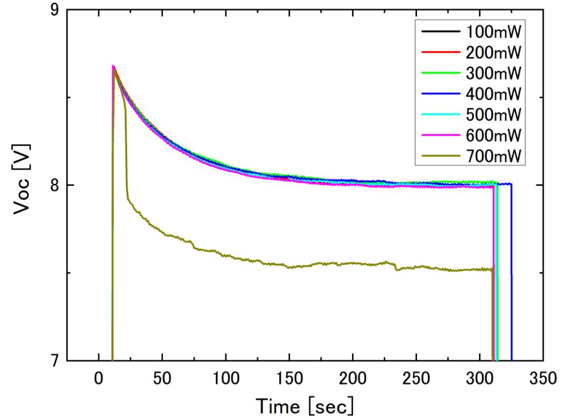
We succeeded in inducing thermal runaway using an artificial shunt spot
