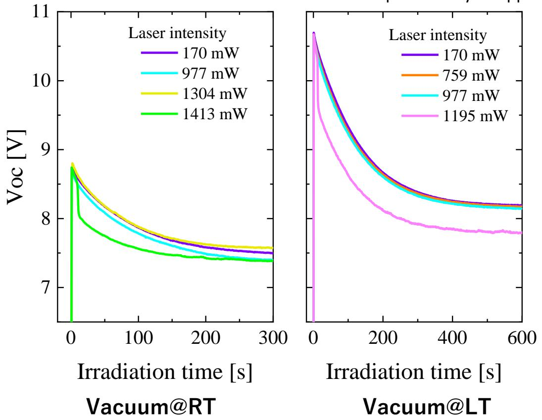
**Thermal runaway easily occurs in a low-temperature environment because temperature difference between the shunt spot and non-shunt region increases when light is irradiated at the low-temperature**
