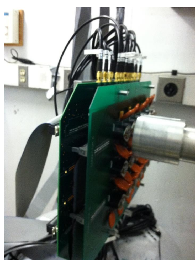
Figure 1: Test PCB inline with beam
