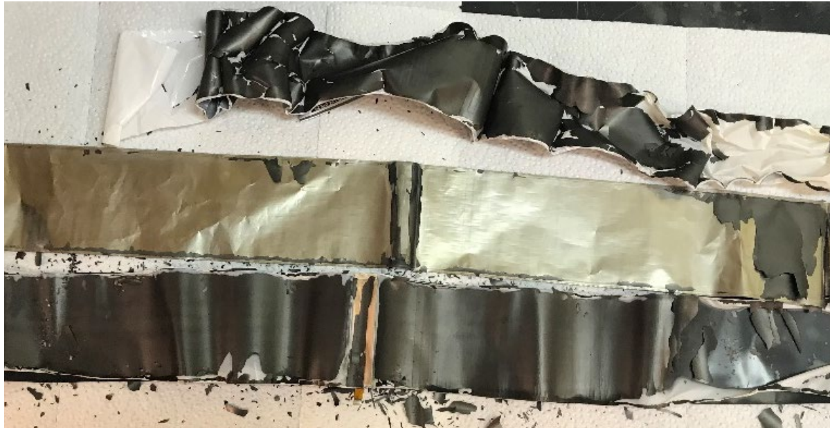
nC-cc1 cell after 465 cycles at 45 °C with 2 x 5-day 0V holds.
