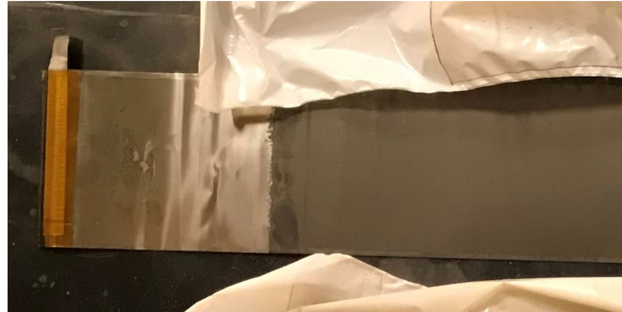
nC-cc2 cell after 1,000 cycles at 45 °C with 5 x 5-day 0V holds.
