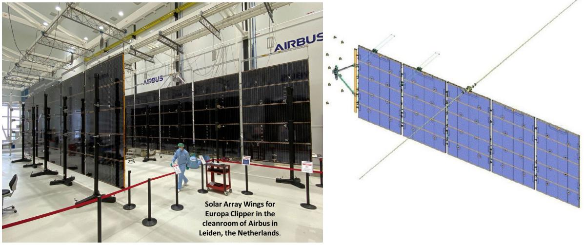
• Wings and antennas are deployable
