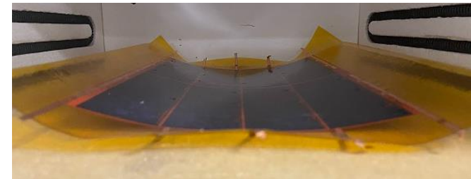
2 mil Kapton HN after thermal treatment at 150°C for 1 hour
