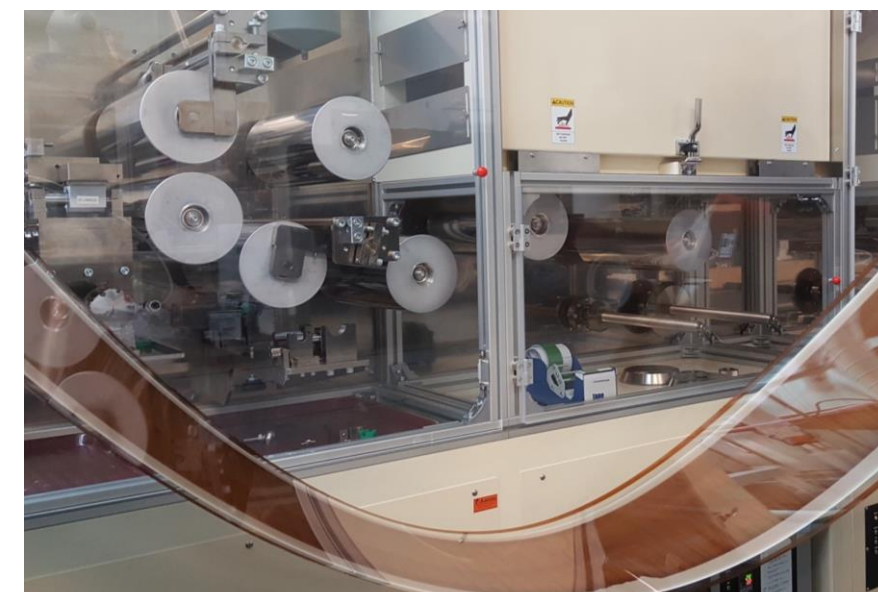
Large-area, roll-to-roll coating on flexible glass—a key technique for low-cost manufacturing
