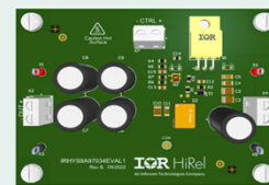
Inrush current limiter evaluation board using the IRHYS9A97034CM.
