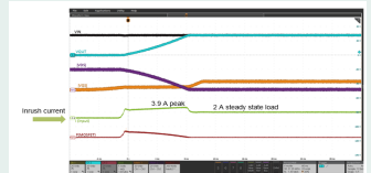
R5 SOA performance in the TO-257AA package limits use to <50-W converters in inrush current limiting applications.
