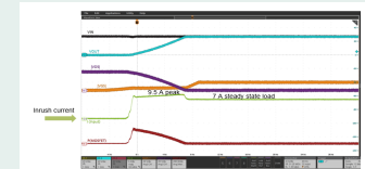
R9 performance in the same package can support >100-W of power dissipation in inrush current limiting applications.
