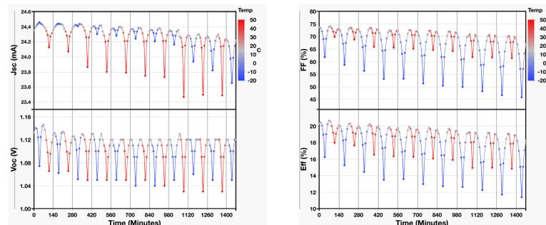
Figure 3. Thermal cycling of unit cell under AM1.5G from -20 °C to 50 °C
