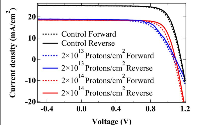
Figure 6. Current Vs. Voltage curves with different proton fluxes
