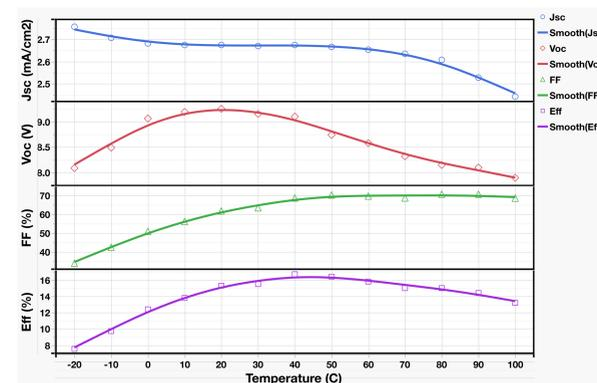
Figure 5. Temperature dependent PV parameters of a mini module (32cm<sup>2</sup>) under AM1.5G from -20 °C to 100 °C
