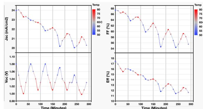
Figure 4. Thermal cycling of unit cell under AM1.5G from 50 °C to 80 °C
