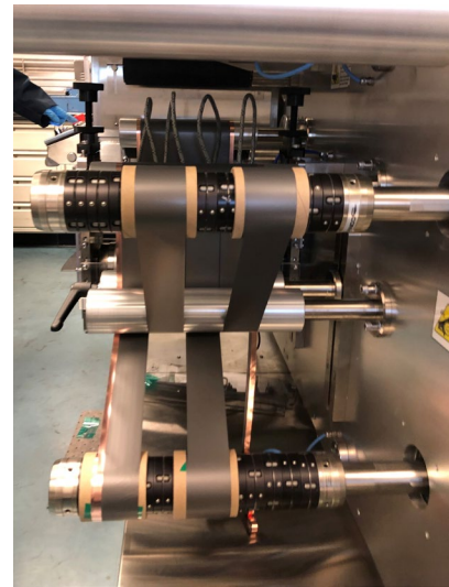
Anode Slitting Process Overview
