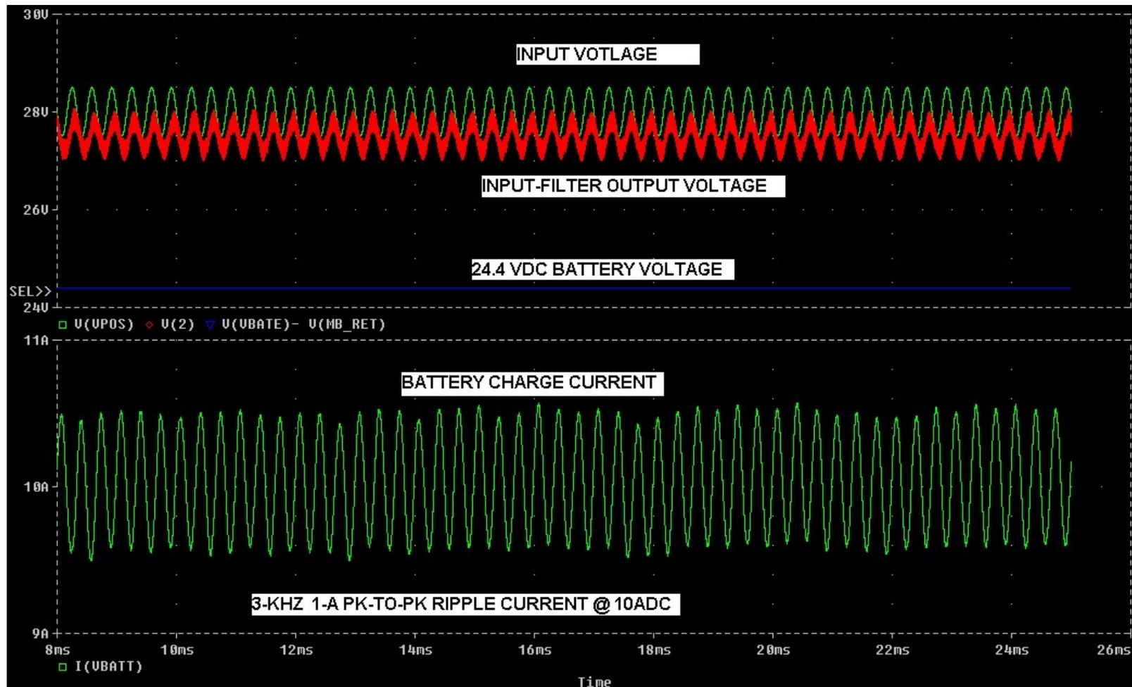
Oscillation @ 3kHz was actually observed from the contractor SV's test data
