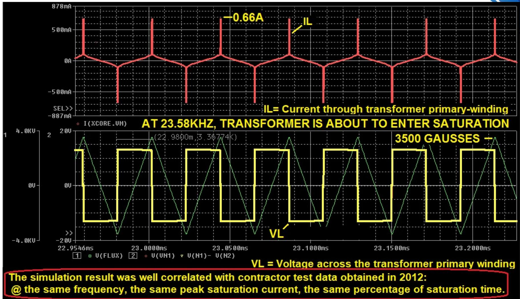
Magnetic saturation is observed from the saturated peak current spike of 0.66 A, which starts at around 23.58 kHz of transformer excitation frequency (square wave of +/-13 V amplitude) as PWM chip's temperature gets warmer.
