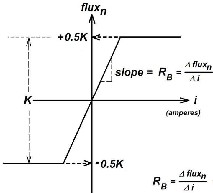
where  $L$  = magnetizing inductance before core saturation
