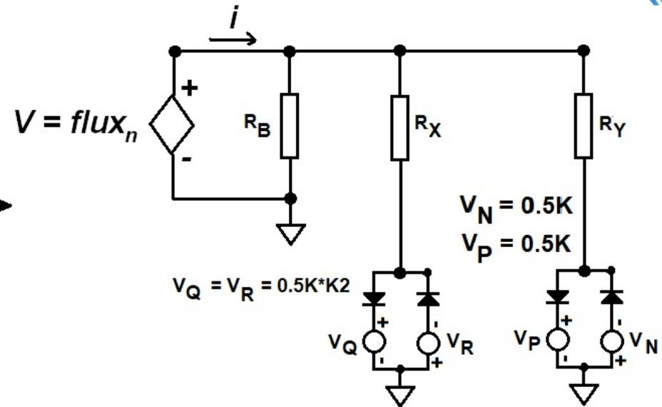
Where  $R_C = \frac{R_X R_B}{R_X + R_B}$       $R_0 = \frac{R_Y R_C}{R_Y + R_C}$       $K_2 = \frac{B_2}{B_m}$
