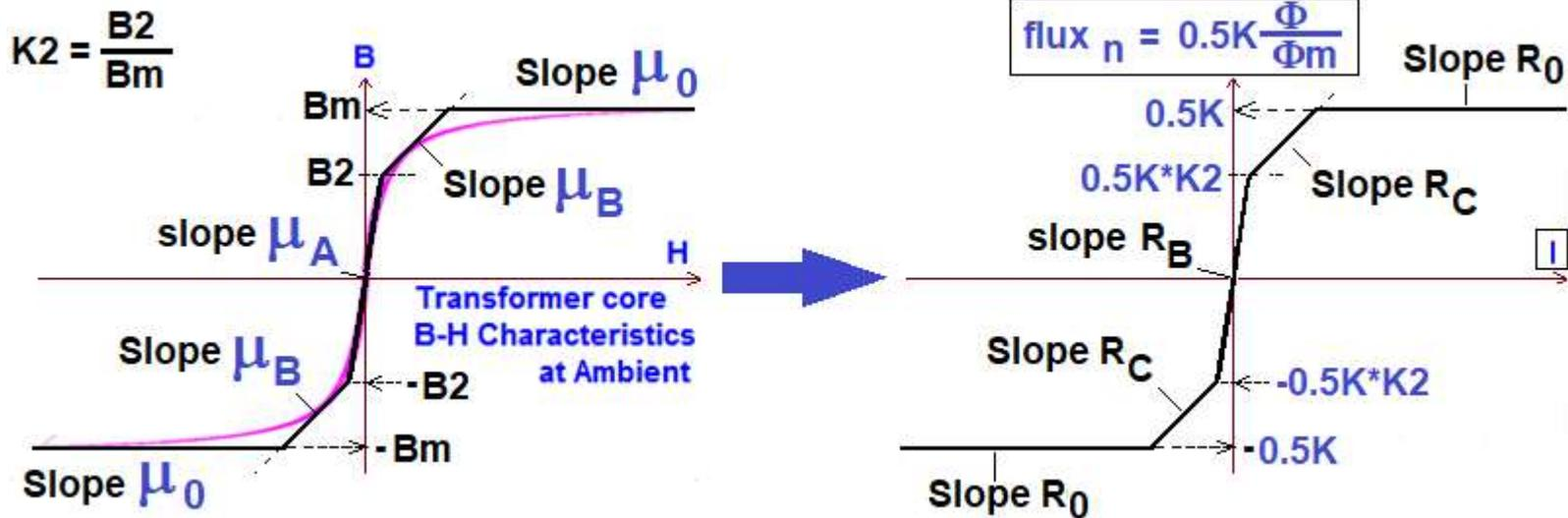
Where slope parameters:  $R_B = \alpha \mu_A$ ,  $R_C = \alpha \mu_B$ ,  $R_0 = \alpha \mu_0$
