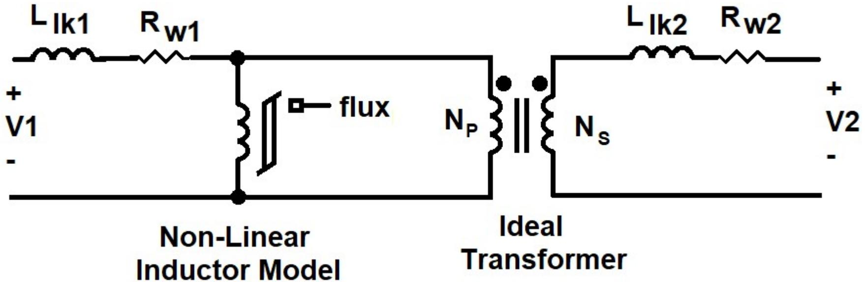
Only one non-linear element contains the magnetic core model. Otherwise, other circuit elements are linear.
