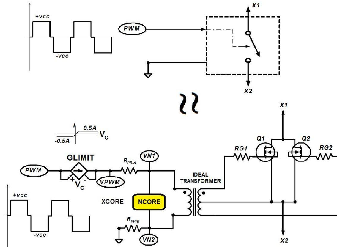
Saturable pulse transformer is decomposed into
