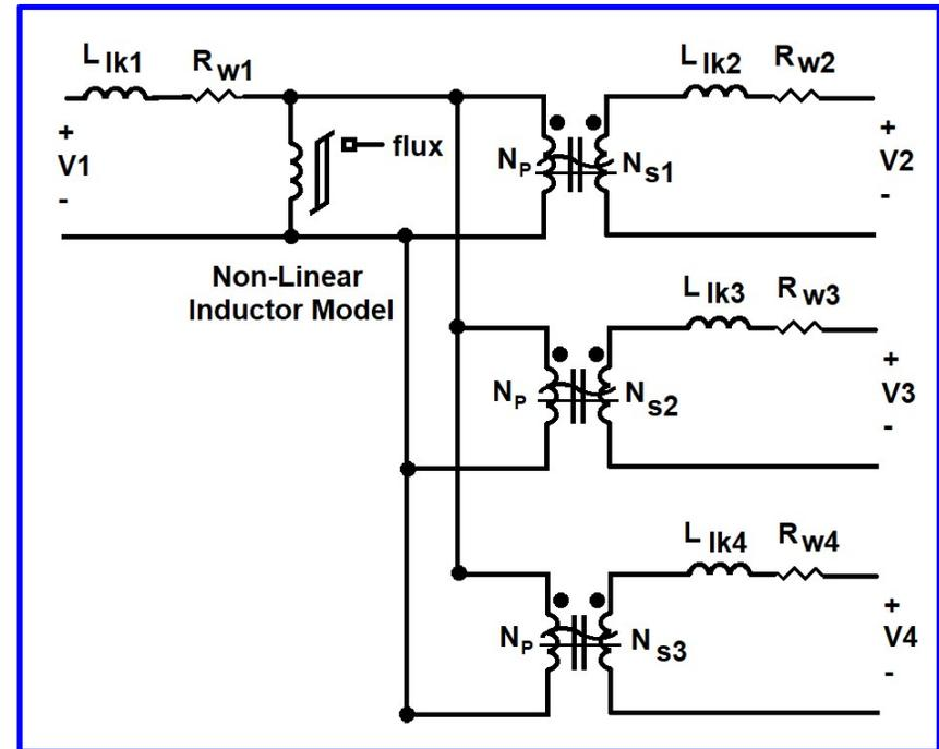
**Only one non-linear model is the core model, otherwise other components are linear and ideal.**
