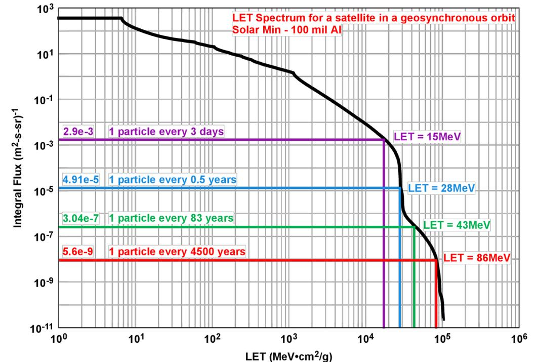
Figure 3: CREME96 LET Spectrum for a Satellite in GEO Assuming Solar Minimum Conditions with 100 mils of Aluminum Shielding
