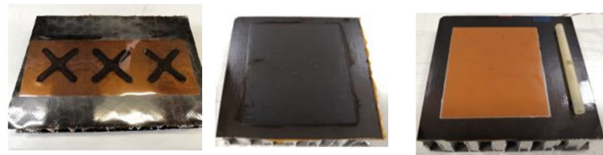
Examples of small coupons for high dose electron irradiation
