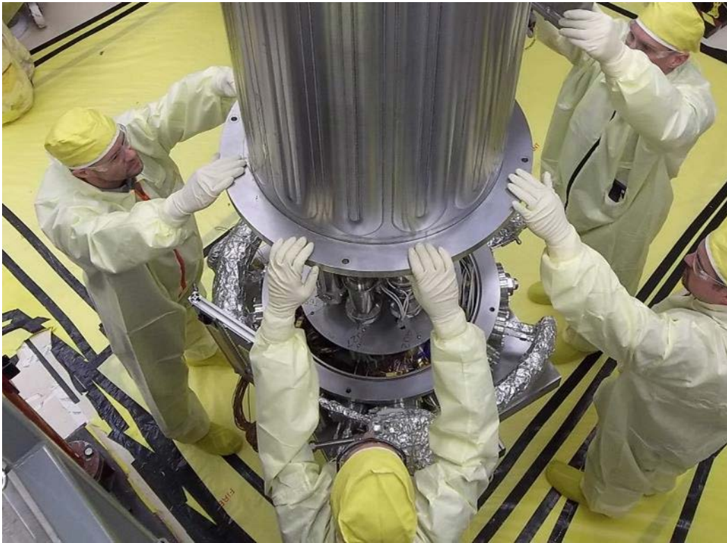
NASA and NNSA engineers lower the wall of the vacuum chamber around the Kilowatt Reactor Using Stirling TechnologY (KRUSTY system). Credits: Los Alamos National Laboratory
