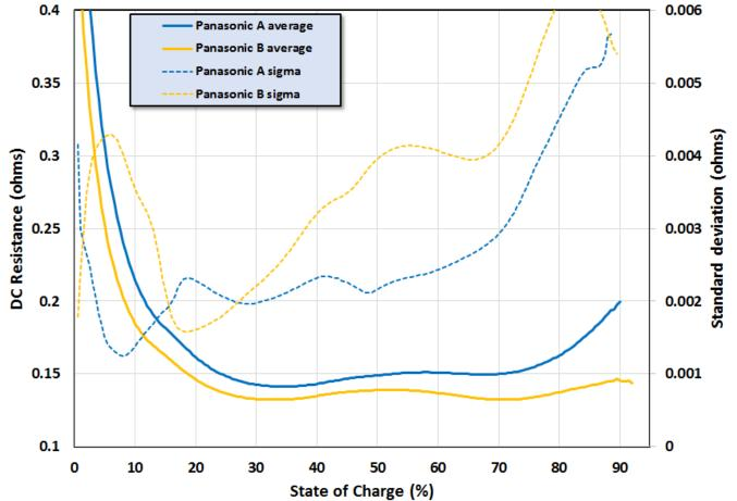
Suggests cell design/manufacturing changes between cell types, and is primary factor in poorer cell statistics for Panasonic B
