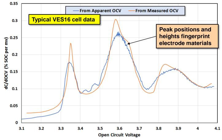
Note: smoothing of voltage data may be needed for differential capacity analysis
