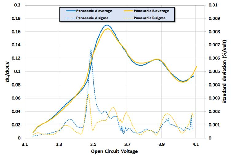
Suggests that a very similar chemistry is used in both of these two cell types
