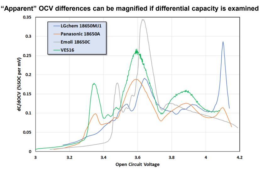
Peaks move around or even disappear for different types of cells, pointing to the detailed signatures of the materials and chemistry used in the cells
