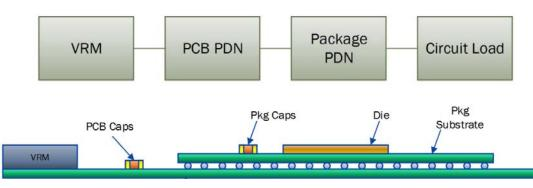
This "REFRENCE DESIGN" resulted in exceeding the allowed voltage deviation by 150% when powering just ONE of FIVE transceivers
