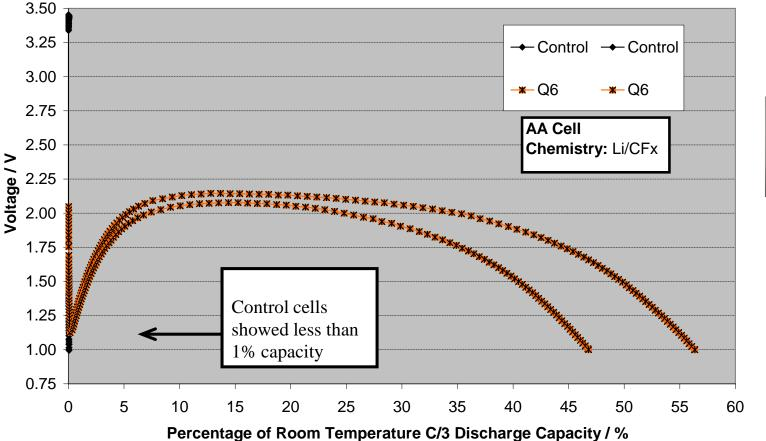
C/3 Discharge at -40°C for Tested Electrolytes
