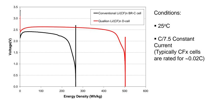
The energy density of the Quallion  $\text{Li}/(CF)_n$  D-cell is about double that of existing  $\text{Li}/(CF)_n$  cells.
