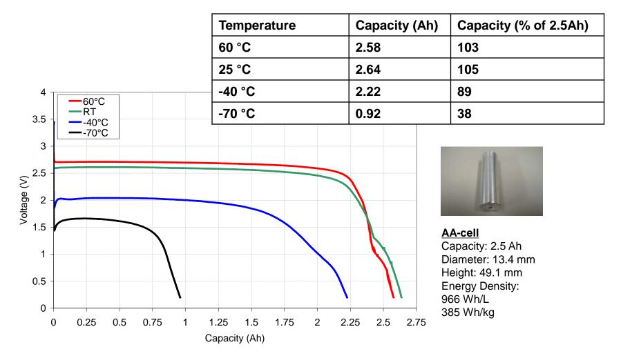
90% capacity at -40°C and 40% capacity retention at -70°C
