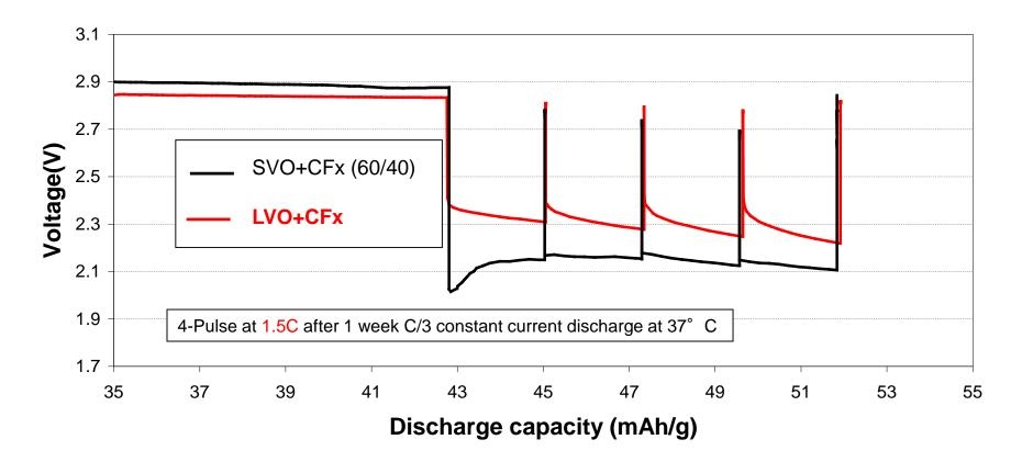
No voltage delay was observed during pulse test
