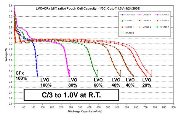
• CFx 100% cells shows no capacity due to the voltage drops below 1.0V at the beginning of discharge
