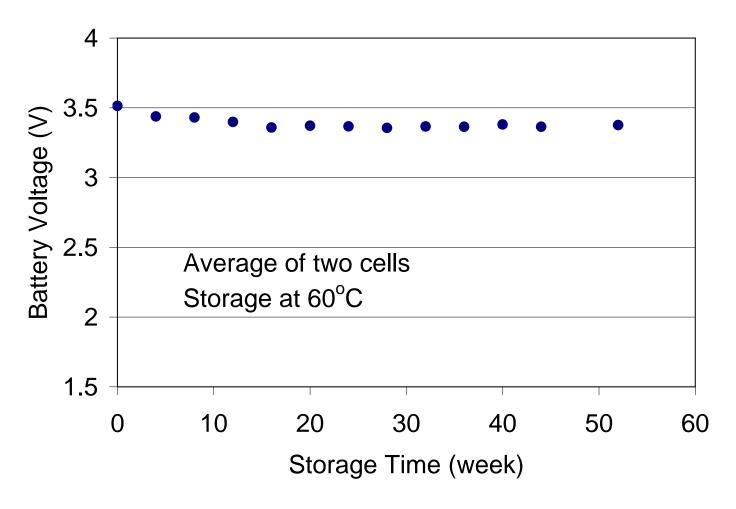
High temperature storage has no effect on the capacity
