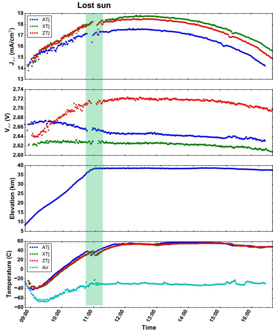
**Stray light baffles are needed for accurate cell characterization**
