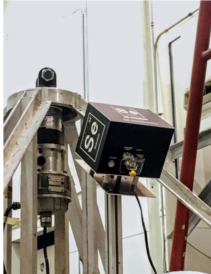
Selenium Payload Mounted at Ft. Sumner on JPL MkIV with protective cover. Power cable charges the battery before flight.
