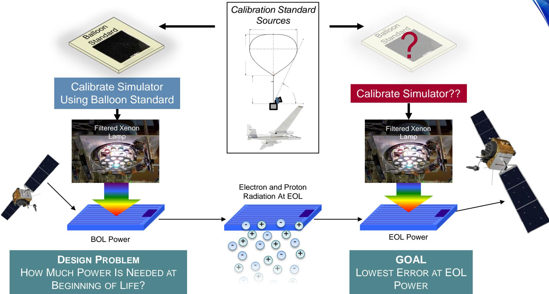
*The challenges associated with predicting EOL performance of multijunction cells require new methods for obtaining calibration standards*
