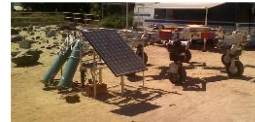
Decoupled RFC demonstration at JPL Mars Yard (fuel cell on ATHLETE + remote hydrogen refueling station)
