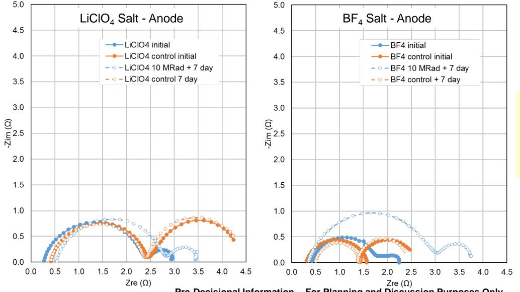
BF<sub>4</sub> salt leads to significant increase in "film" resistance on anode
