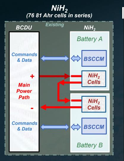
BCDU: Battery Charge / Discharge Unit BIU: Battery Interface Unit BSCCM: Battery Signal Conditioning and Control Module
