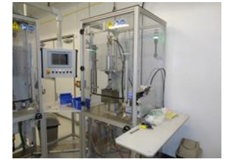
Grooving and sealant application station
